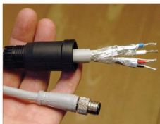
Left —In networking, heavy or light cable and connectors are necessary, depending on the amperage requirements of the devices to be connected to a given system. Below —Note the relative difference in the heavy and light connectors used with the two different sizes of NMEA 2000 cable.
