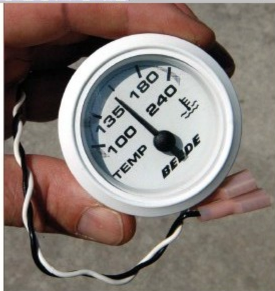
A temperature gauge converted to operate on an E-Plex system. The twisted wires will be the only connection.
