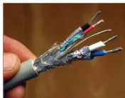
NMEA 2000 heavy cable is really a bundle of five smaller cables: two for data, two for power, and one ground wire.
